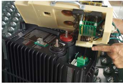
using Pogo-Pins, LED sensors & Bus Bars
