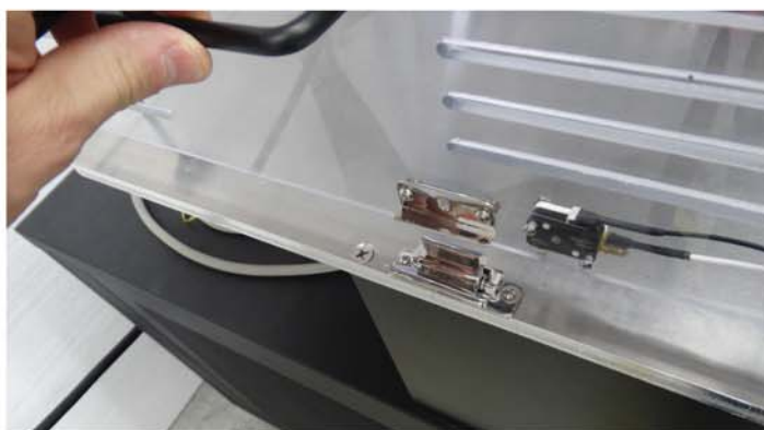
Safety Cover MicroSwitch and Latch
