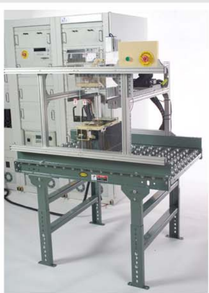
Front view of System with Inverter Test Fixture and a UUT
