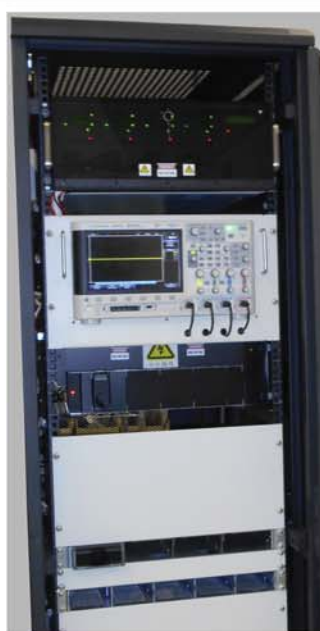
Fixture with added HV Loads and Scope
