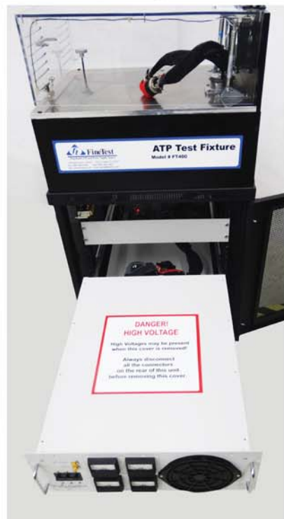
Pull-out Interface Unit for easy Maintenance, and Service
