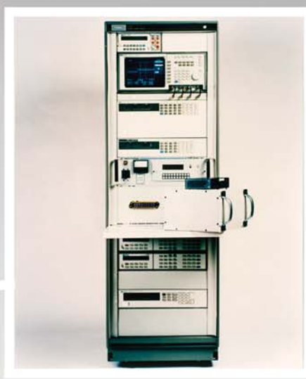
Plug-In UUT Test Fixture
