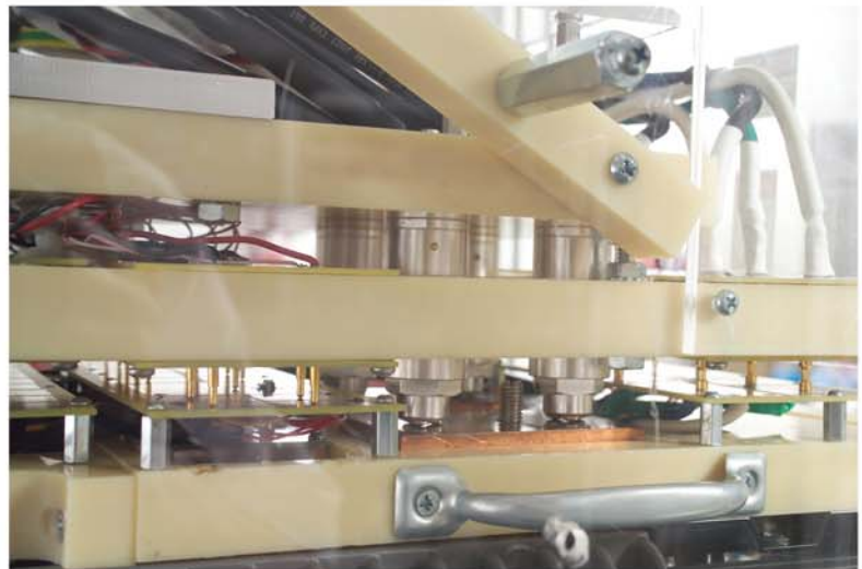
Close-Up of High Current Pogo-Pins
