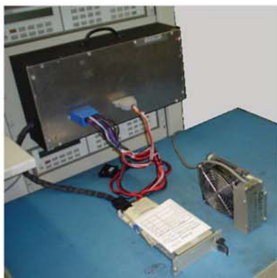
Cable to UUT Test Fixture
