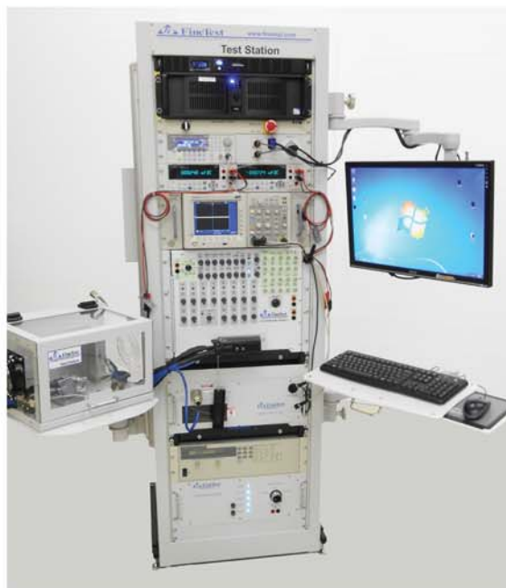
ITA mounted on height adjustable arm
