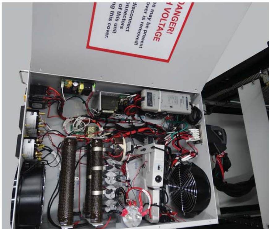
Interface Unit with Top Removed showing Differential and Current Probes, Resistive Loads, Relays etc.
