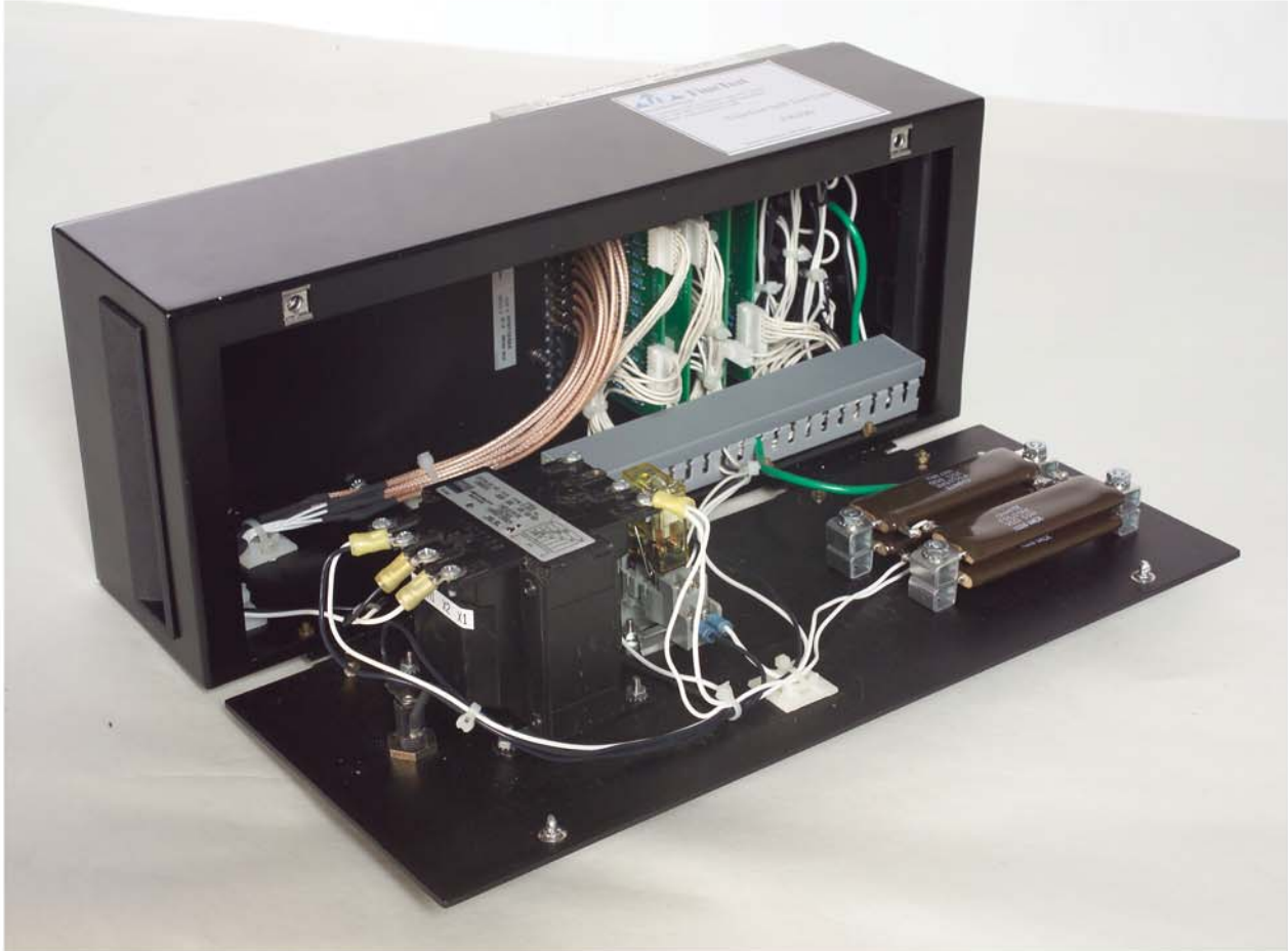
Self-Test Fixture with rear cover open
